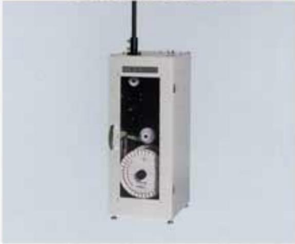
Can supply wire electrodes continuously for long periods (20kg bobbin wire). Supports 0.2, 0.25 and 0.3 diameter wires.
