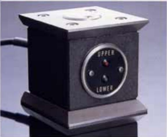
By setting the jig on the table and touching the wire with its edges, the verticality of wire electrode against the table can be automatically detected corrected.
