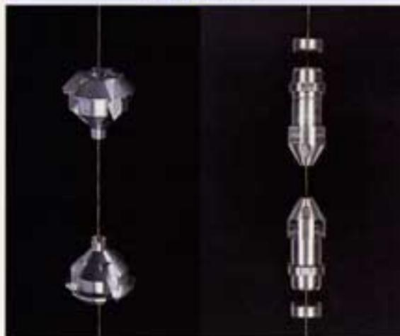
Wire die guides provided for 0.1, 0.15, 0.2, 0.25 and 0.3 diameter wires, supporting a wide range of applications.
