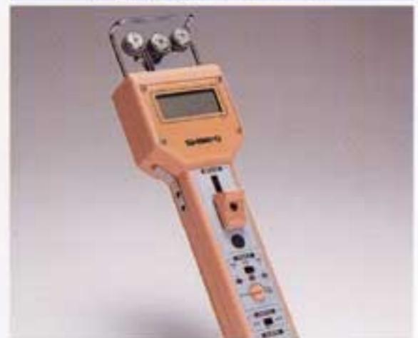
High performance meter with an accuracy of  $\pm 1.5\%$  (fullscale). Measurement range : 200 to 2,000 gf.
